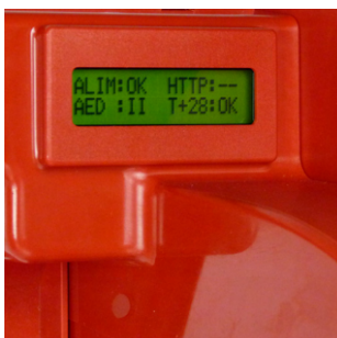
LCD screen displaying general status or incidents : power, network, AED, temperature
