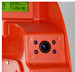
Infra-red lens taking pictures upon the opening of the cabinet and removal of the AED
