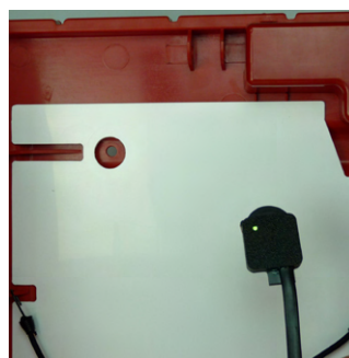
Sensor to assist the remote monitoring of the AED status, temperature, and presence.
